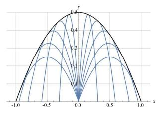
**Figure 2.** The black curve is the envelope, the families of the parabolic trajectories are in blue.
