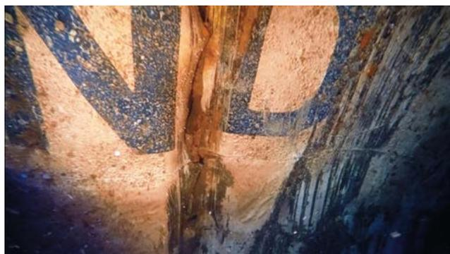
**Figure 7.** Vertical crack/rift of Deck #4 located at the transversal frame #138 on the port side (left side).
