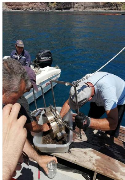
**Figure 8.** Grab sampler in action collecting seabed sediment (Thira island).
