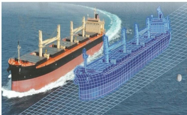
**Figure 1.** The ship and her digital twin. Source: ClassNK (modified) 2019; a digital twin is a reproduction of a ship simulating her movement and operational condition and can make predictions about her.
