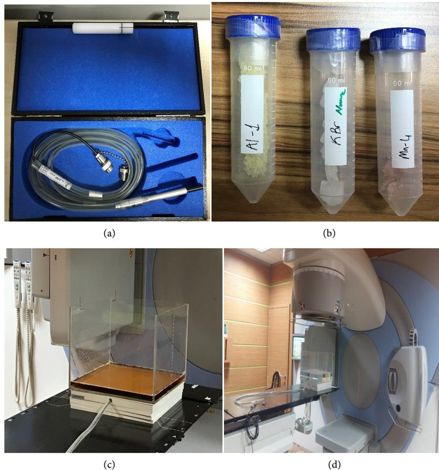
**Figure 2.** The FC65P ion chamber (a), some of the elements used in this study (b), experimental setup for iron (c) and water (d).
