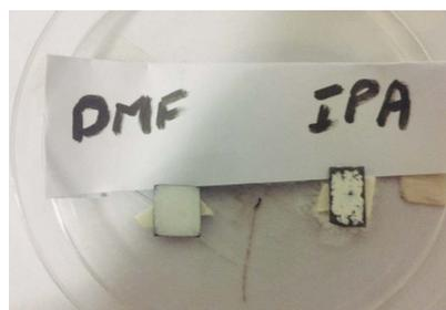
**Figure 2.** Shows Exfoliated h-BN in DMF and IPA drop-casted on Silicon Substrate.
