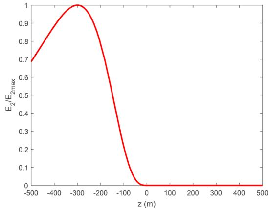
**Figure 2.** The curve  $E_z/E_{z,max}$  for a free electron beam propagating in a linear range of about 1000 meters.
