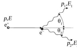
**Figure 6.** Energy and momentum of the positron-electron annihilation in flight.
