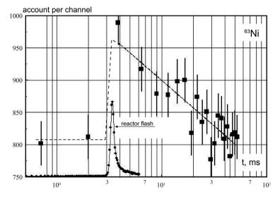
**Figure 3.** The result of the accumulating registration of beta-electrons emitted by <sup>63</sup>Ni. Measurement time is 1 day. The level of amplitude discrimination close to the boundary energy was chosen experimentally. On abscissa: time in ms in the logarithmic scale.
