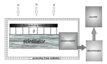
Figure 2. Diagram of the measuring unit.
