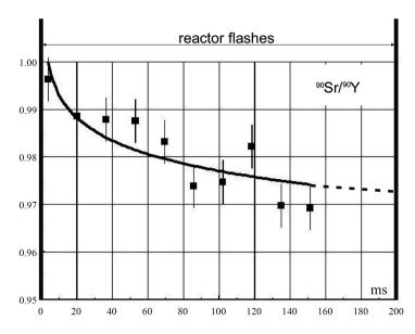
**Figure 1.** The result of the accumulation of registered beta-electrons emitted by the <sup>90</sup>Sr/<sup>90</sup>Y source in the time interval between reactor flashes.
