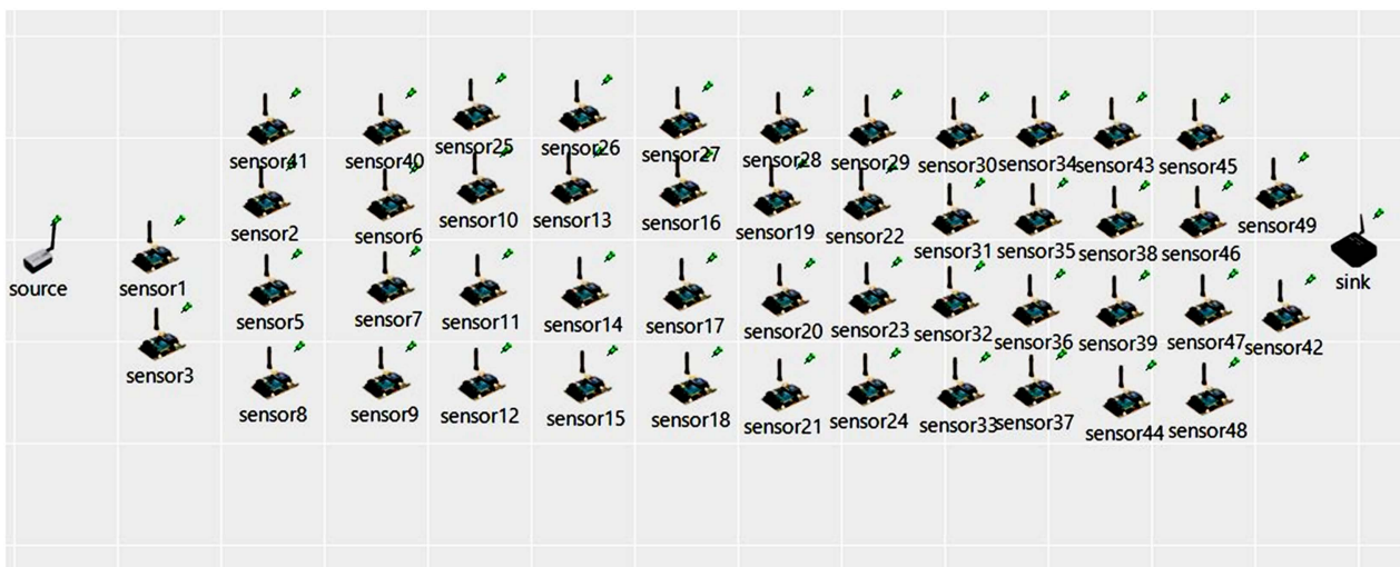
Figure 3. Network topology with 50 nodes in OMNeT++ simulator.
