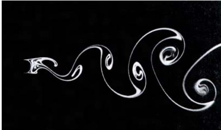
**Figure 1.** Karman vortex downstream of circular cylinder.
