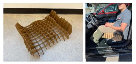
Figure 16. Version 2: Low-fidelity seat mapping model and testing.
