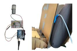
Figure 17. Air pump side bolster.
