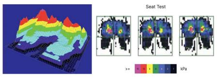
Figure 11. Car seat pressure distribution.
