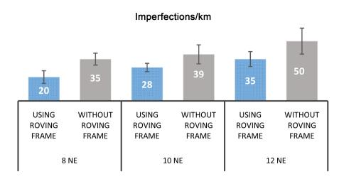
Figure 4. Influence of roving frame on IPI.
