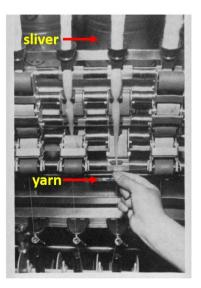
**Figure 2.** Ring frame producing yarn directly from sliver [5].
