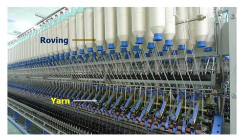
Figure 1. Ring frame producing yarn from roving.
