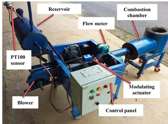
**Figure 2.** Pictorial view of the WLO burner system.
