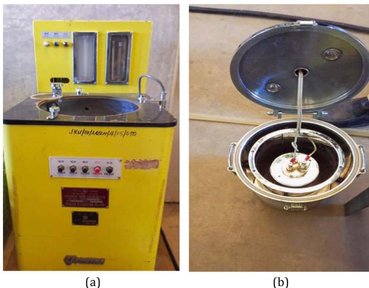
**Figure 3.** Adiabatic bomb calorimeter; (a) The front view of the adiabatic bomb calorimeter, (b) Pictorial view of the inner components of the adiabatic bomb calorimeter.
