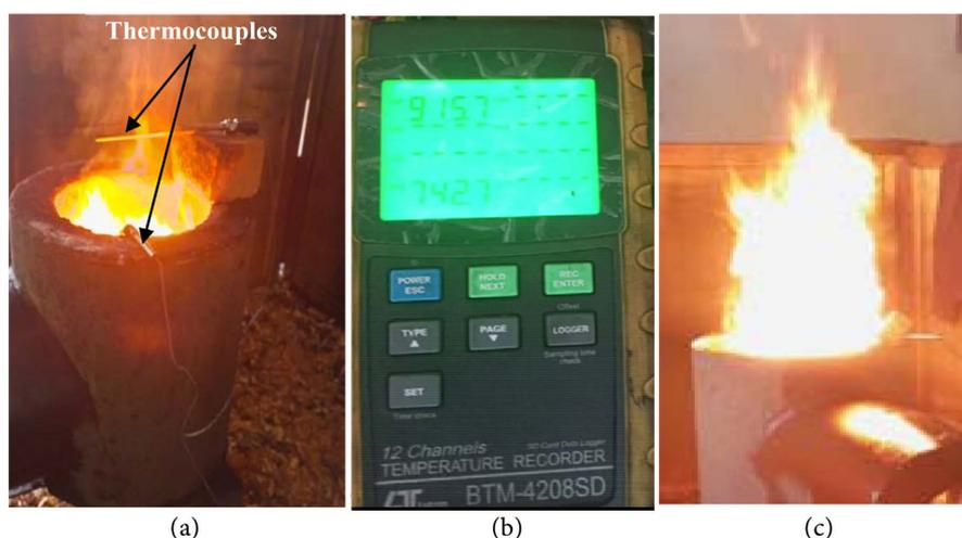
**Figure 5.** Flame temperature measurements; (a) Thermocouple setting for temperature detection, (b) Flame temperature captured by data logger, (c) Flame obtained from the burner.
