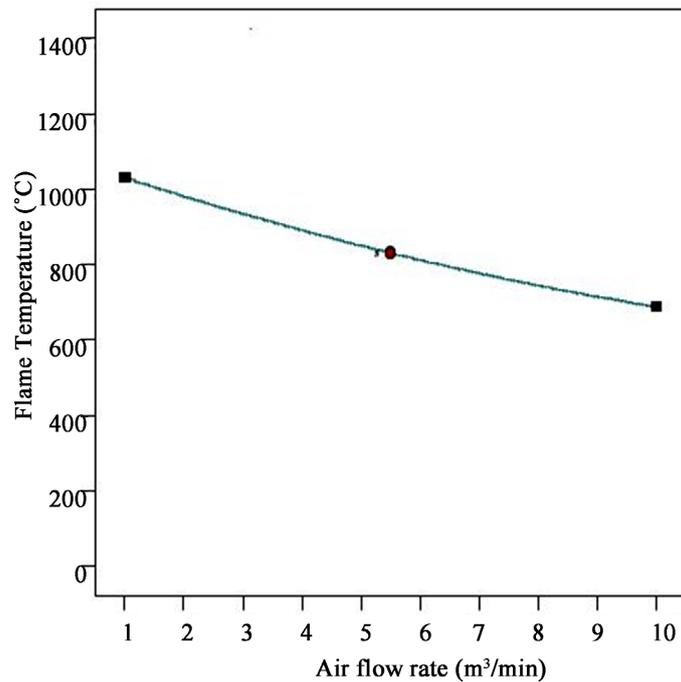
**Figure 6.** Effect of air flow rate on flame temperature.
