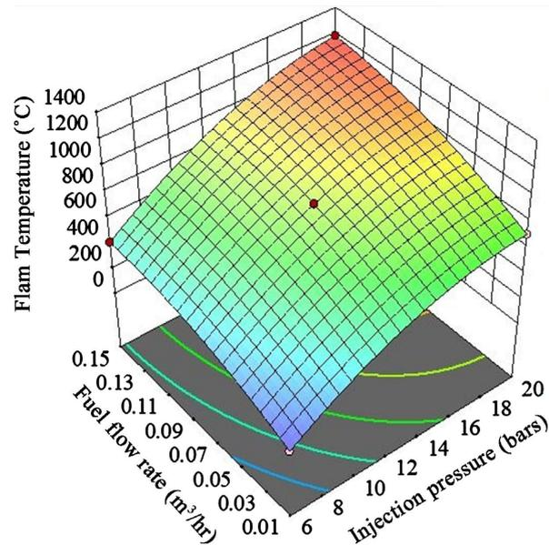
**Figure 9.** Effect of fuel flow rate and injection pressure on flame temperature.
