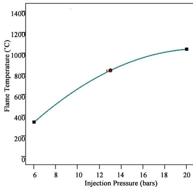
**Figure 7.** Effects of injection pressure on flame temperature.
