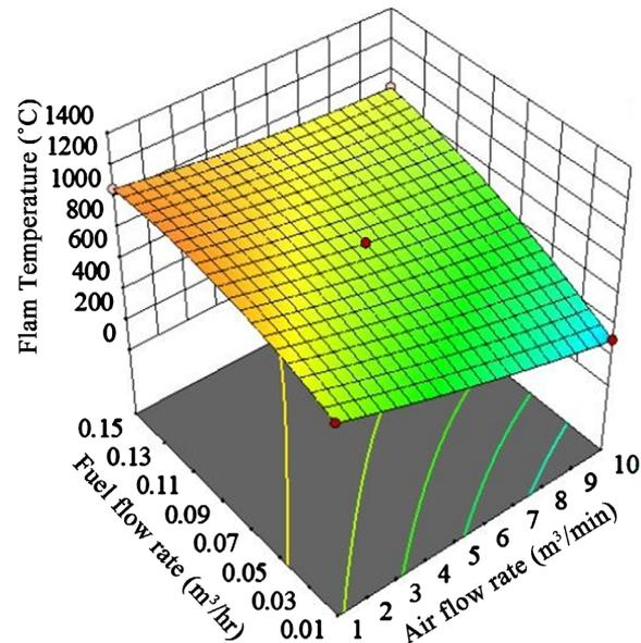
**Figure 11.** Effect of fuel flow rate and air flow rate on flame temperature.
