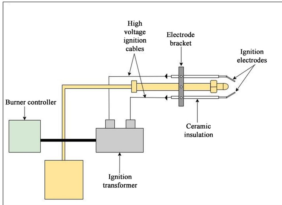
**Figure 4.** Fuel auto-ignition set-up.
