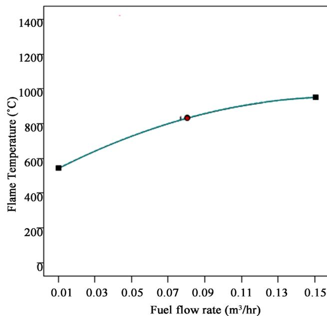
**Figure 8.** Effect of fuel flow rate on flame temperature.
