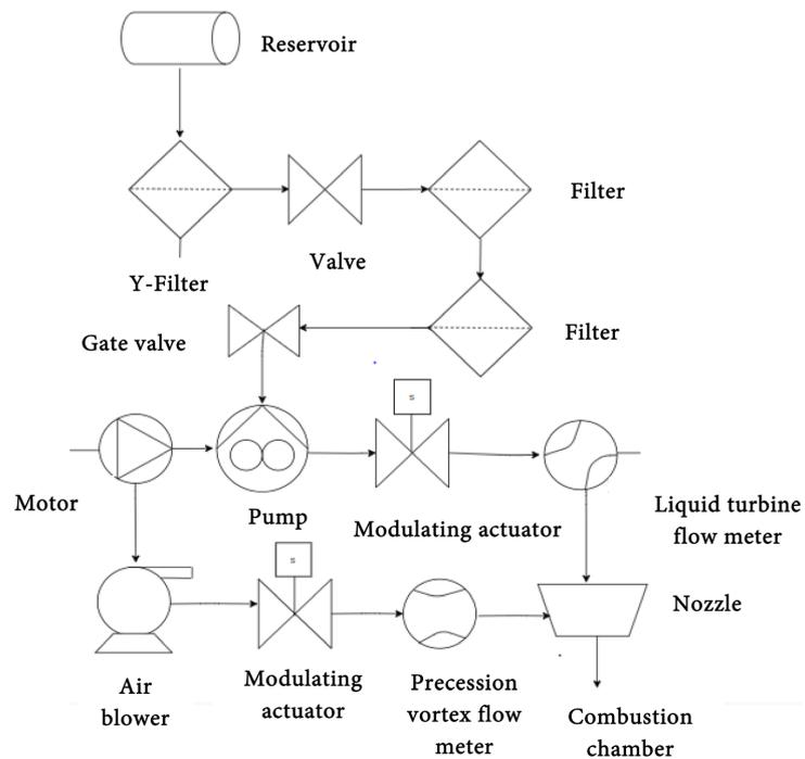
**Figure 1.** Schematic diagram of the WLO burner.
