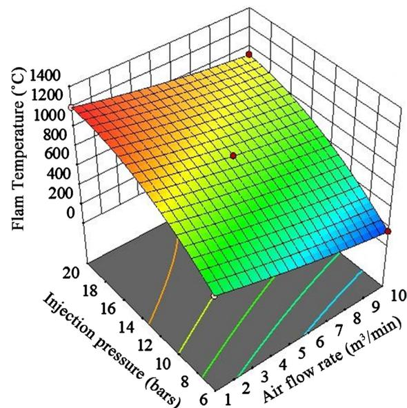
**Figure 10.** Effect of air flow rate and injection pressure on flame temperature.
