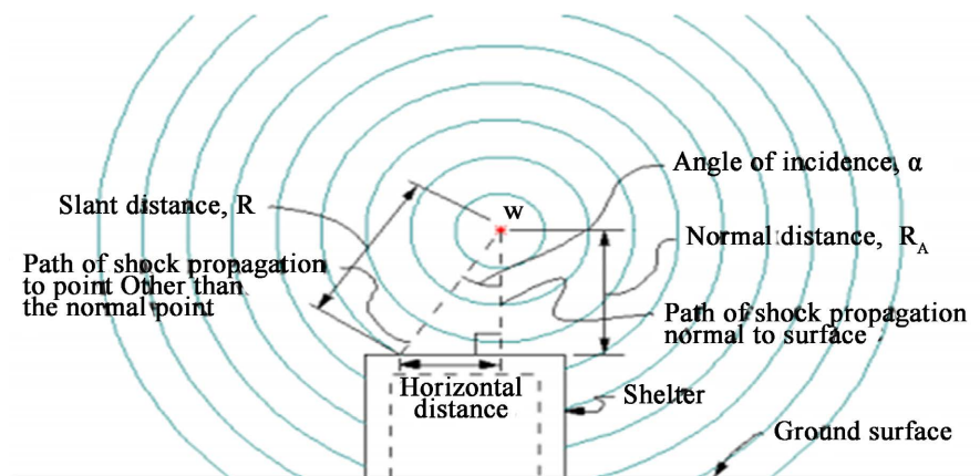
Figure 1. Free air burst wave front [44].
