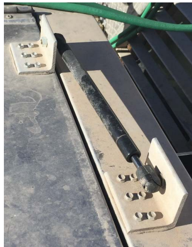
Figure 7. Pneumatic strut in a closed position on a fish transport tank.
