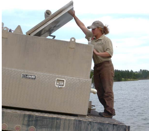
Figure 4. An example of a folding lid stay hinge unable to be fully raised to a locked open position.
