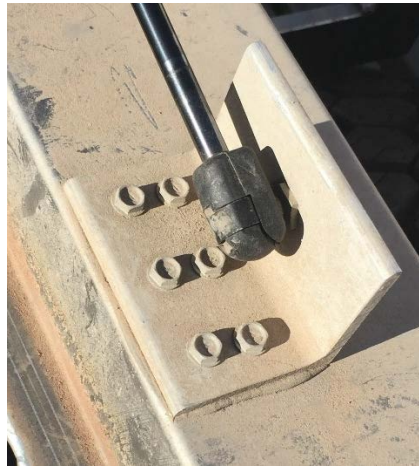
Figure 8. Attachment of a pneumatic strut to a fish transport tank using aluminum angle.
