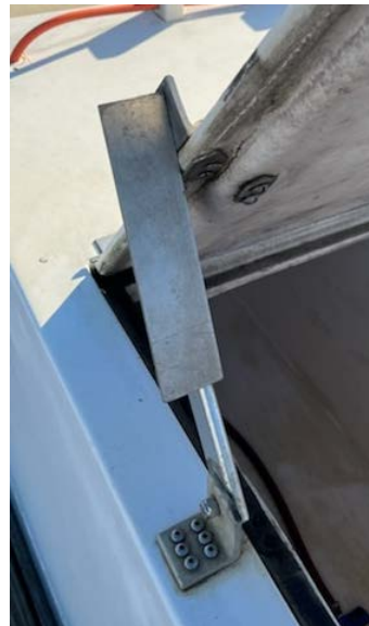
Figure 1. Photograph of a typical folding lid stay hinge on a fish transport tank.
