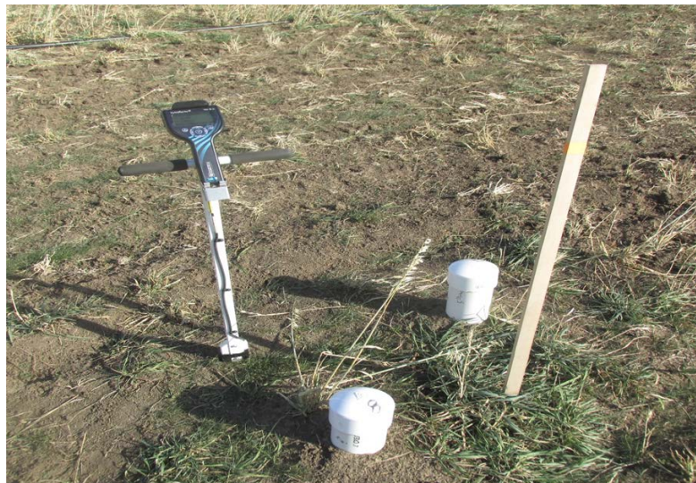
Figure 5. Hydro sense II moisture instrument and monitoring wells.
