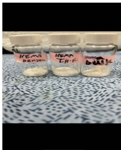
Figure 12. Homopolymerization of HEMA after dried in a vacuum oven 24 hours.
