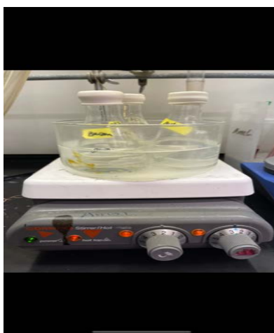
Figure 9. Homopolymerization of styrene in silicon oil bath at 60°C for 24 hours.
