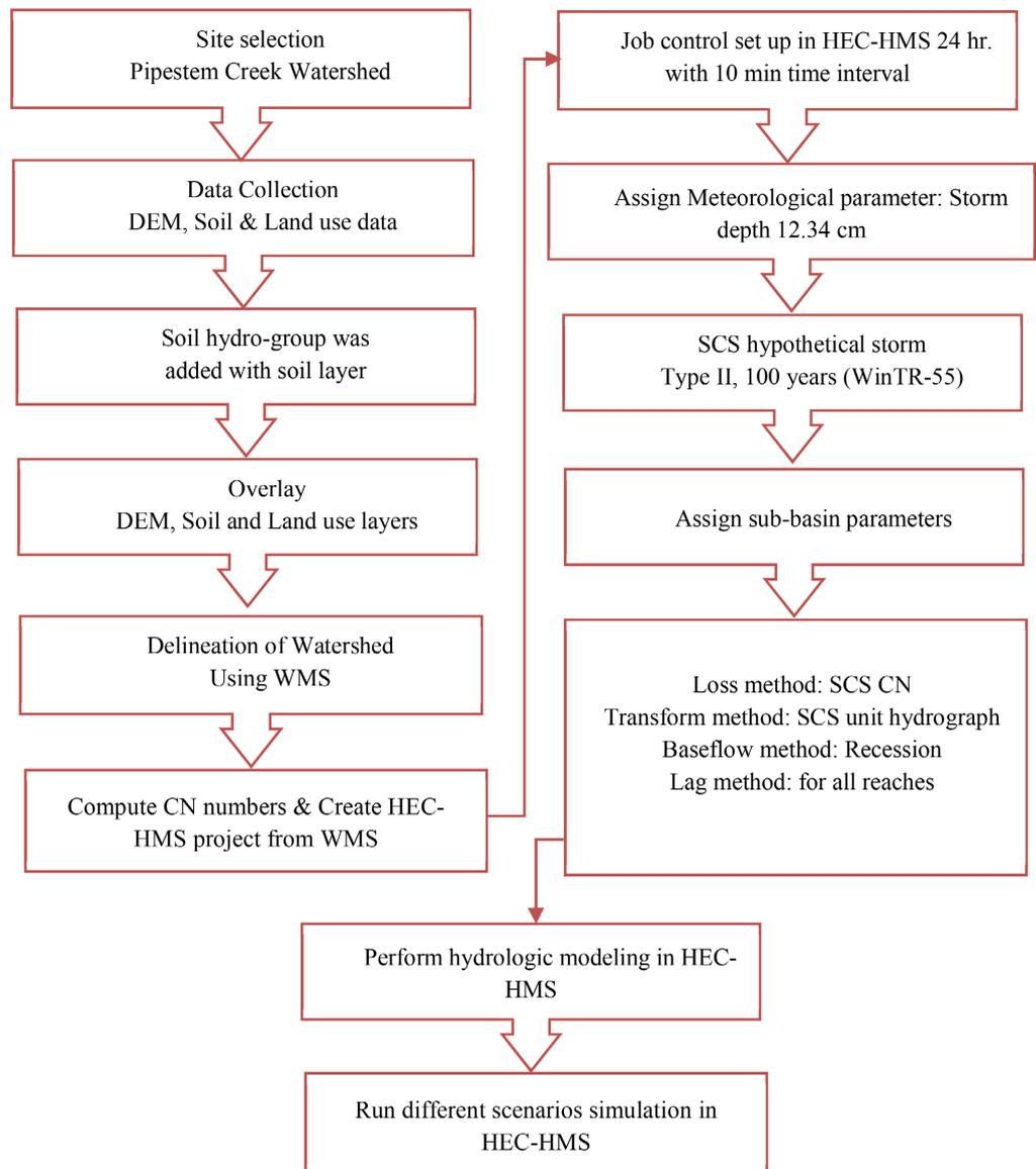
**Figure 2.** Flow chart of the modelling process.
