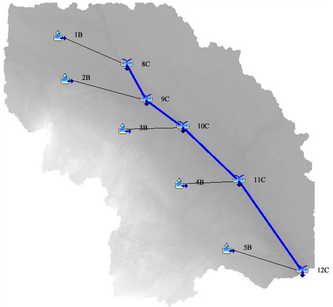
**Figure 4.** Layout of the HEC-HMS model.
