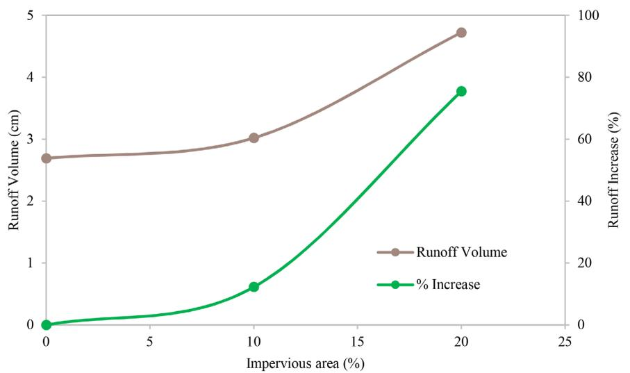
Figure 9. Effect of impervious area on runoff volume.
