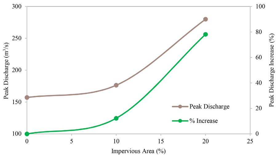
Figure 8. Effect of impervious area on peak discharges.
