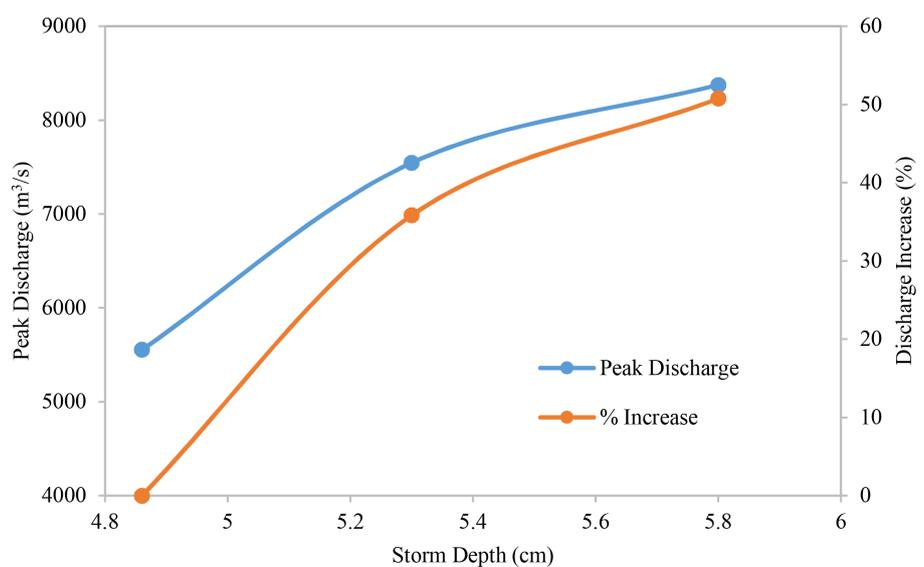
**Figure 6.** Effect of increasing storm depths on peak discharges.
