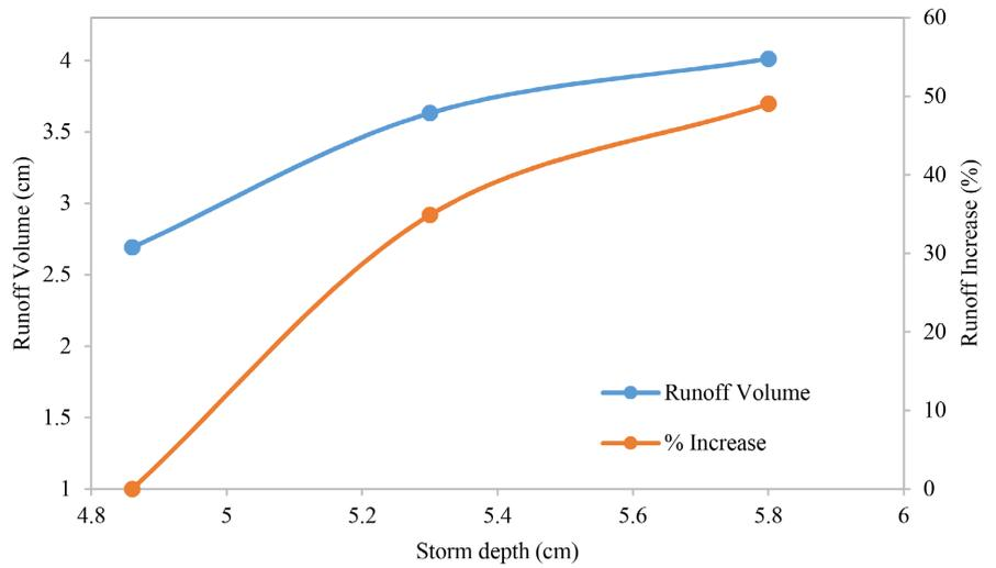
Figure 7. Effect of increasing storm depths on runoff volume.
