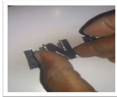
Figure 8. Pressing the texts on the porcelain.
