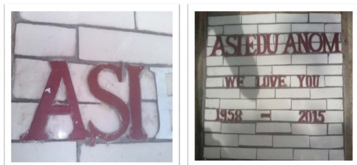
Figure 5. Sticker removed to expose the coated Aluminium text.
