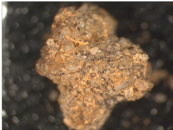
**Photo 15.** Microphotograph of a quartz grain conglomerate with ochre cement.
