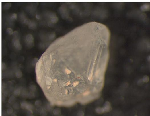
**Photo 8.** Microphotograph of a blunt quartz grain with a large dissolution dihedral.
