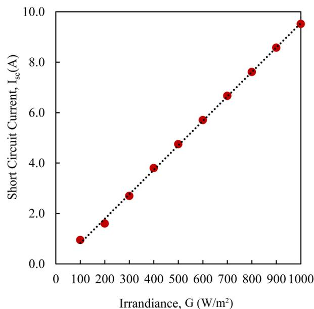
**Figure 4.**  $I_{sc}$ -G curve of monocrystalline PV module.
