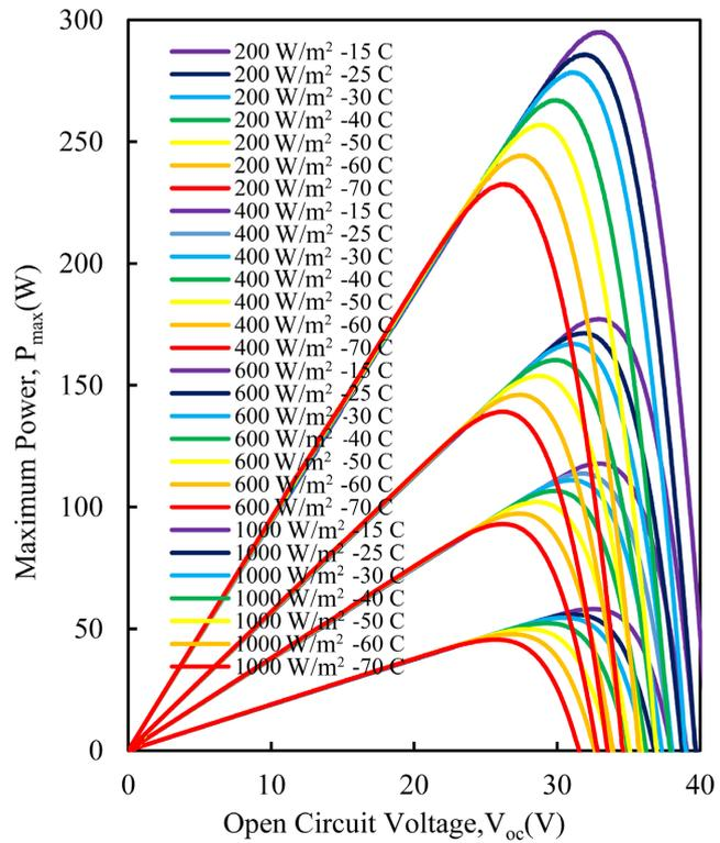
**Figure 7.**  $P_{max}$ -  $V_{oc}$  measurements of monocrystalline PV module at various irradiance levels.
