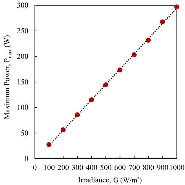
**Figure 5.**  $P_{\max}$ - $G$  curve of monocrystalline PV module.
