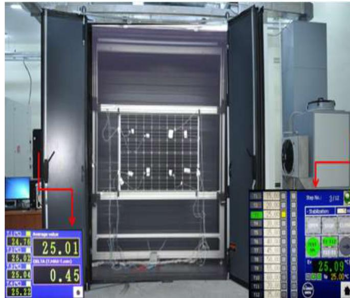
**Figure 1.** Thermal chamber integrated solar simulator system.
