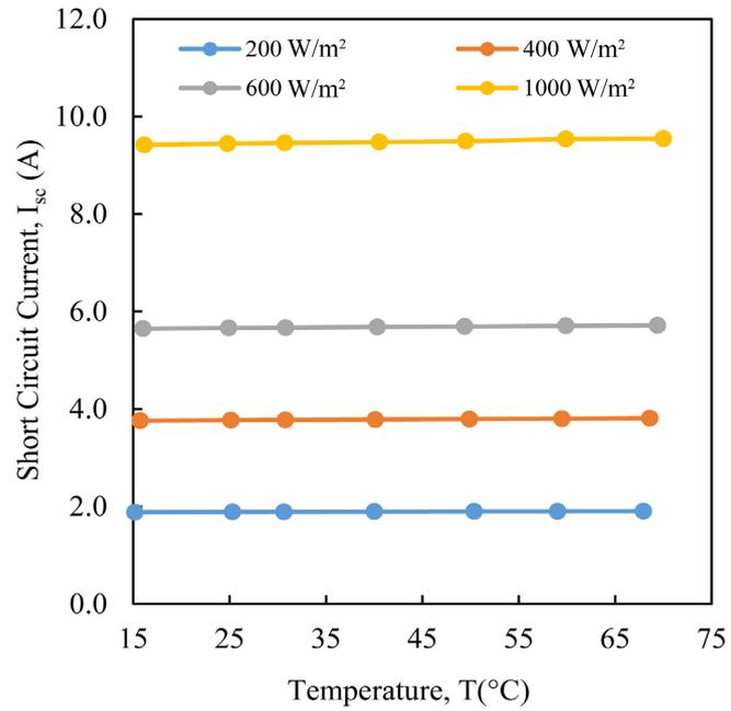
**Figure 8.**  $I_{sc}$ - $T$  graph of monocrystalline PV module at various irradiance levels.
