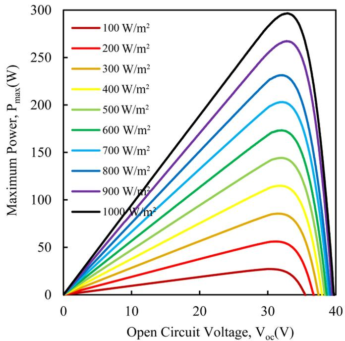
**Figure 3.**  $P_{max}$ -  $V_{oc}$  curves of monocrystalline PV module.
