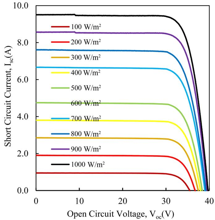
**Figure 2.**  $I_{sc}$ -  $V_{oc}$  curves of monocrystalline PV module.
