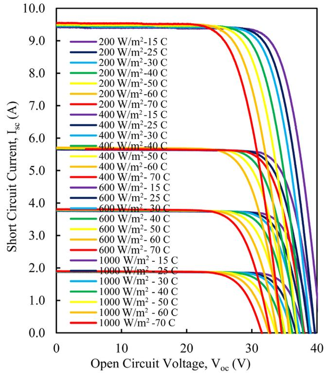
**Figure 6.**  $I_{sc}$ -  $V_{oc}$  measurements of monocrystalline PV module at various irradiance levels.
