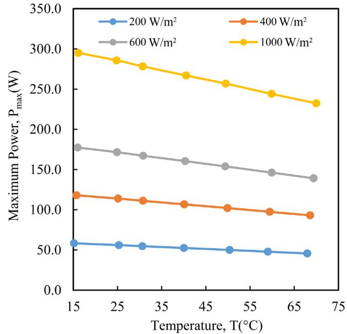
**Figure 10.**  $P_{\max}$ - $T$  graph of monocrystalline PV module at various irradiance levels.
