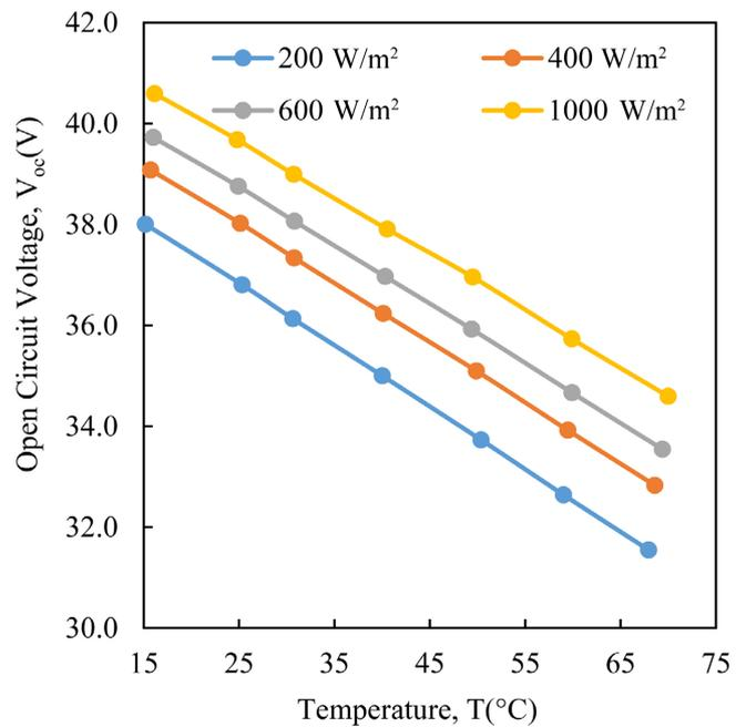
**Figure 9.**  $V_{oc}$ - $T$  graph of monocrystalline PV module at various irradiance levels.
