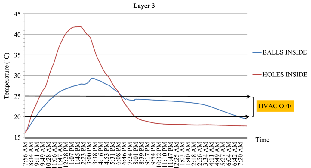
Figure 3. The styrofoam layers, one filled with PCM spheres and the other with holes, during the transient heat mode in the summer, at position 3 in the gypsum wall.
