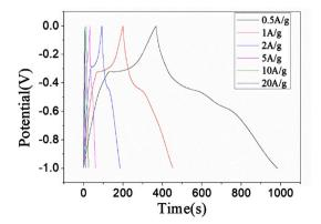
Figure 4. GCD curves of SPCF/MnO<sub>2</sub>-2.0 at various current density.
