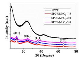
Figure 1. XRD patterns of SPCF and SPCF/MnO<sub>2</sub> composites.
