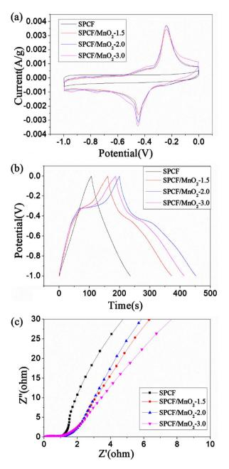
**Figure 3.** CV curves at scan rate of 5 mV/s (a), GCD curves at 1 A/g (b), and Nyquist plots (c) of SPCF and SPCF/MnO<sub>2</sub> composites.
