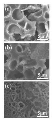
**Figure 2.** SEM images of SPCF/MnO<sub>2</sub>-1,5 (a), SPCF/MnO<sub>2</sub>-2.0 (b), and SPCF/MnO<sub>2</sub>-3.0 (c).
