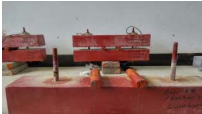
Figure 2. Paired beams before submerged.
