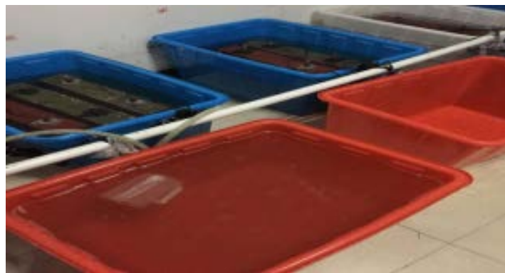
Figure 3. Beams exposed into NaCl solution.
