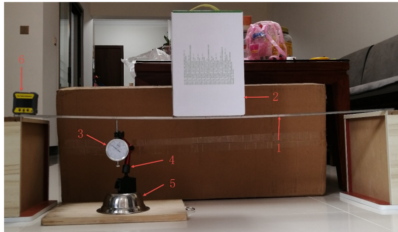
Figure 4. Experimental setup. (1-simply supported steel beam, 2-load, 3-dial indicator, 4-support, 5-base, 6-inclinometer).
