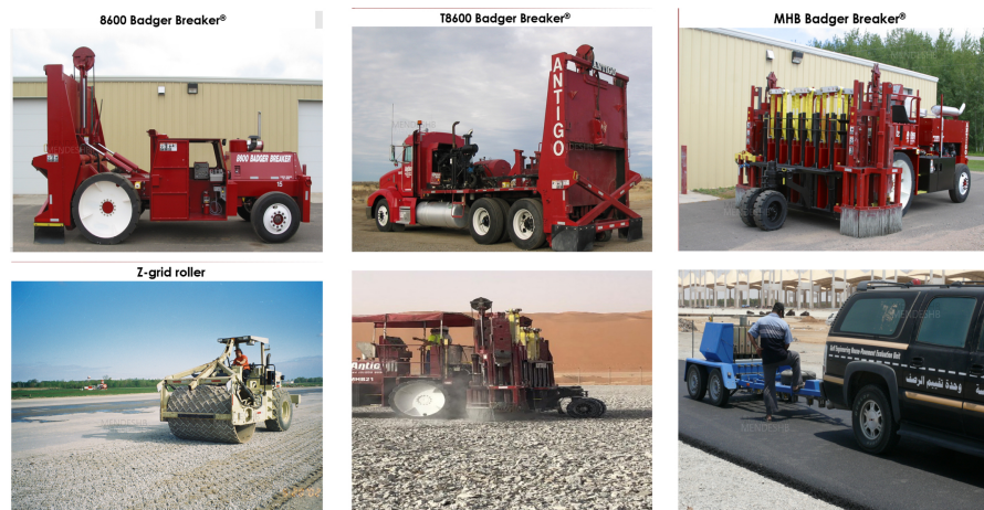
Figure 3. Equipment used for the execution and quality control of rubblization (courtesy from Antigo construction inc. and gulf engineering house).
