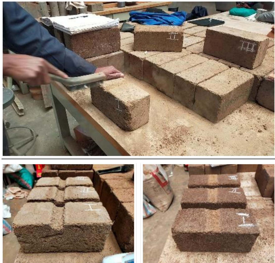
Figure 3. Conducting an abrasion test on the blocks.
