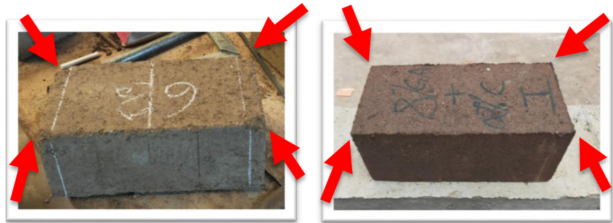
Figure 6. Pictures showing the edges of the blocks without GA (on left) and with GA (on right).
