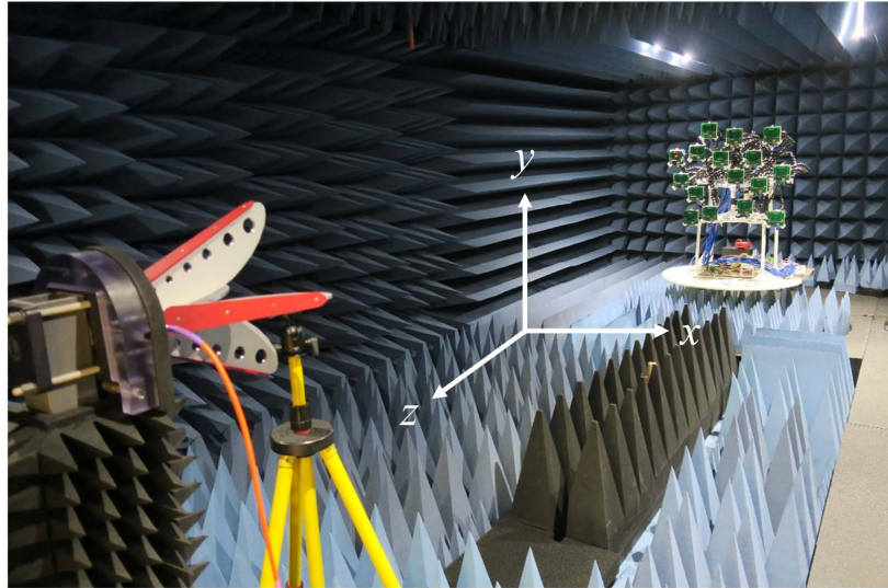
Figure 8. The photograph of the sixteen-element experimental array displaced in the anechoic chamber.
