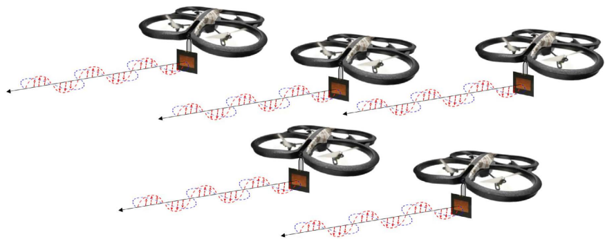
Figure 1. A wireless phased array beamforming system carried out by drones.
