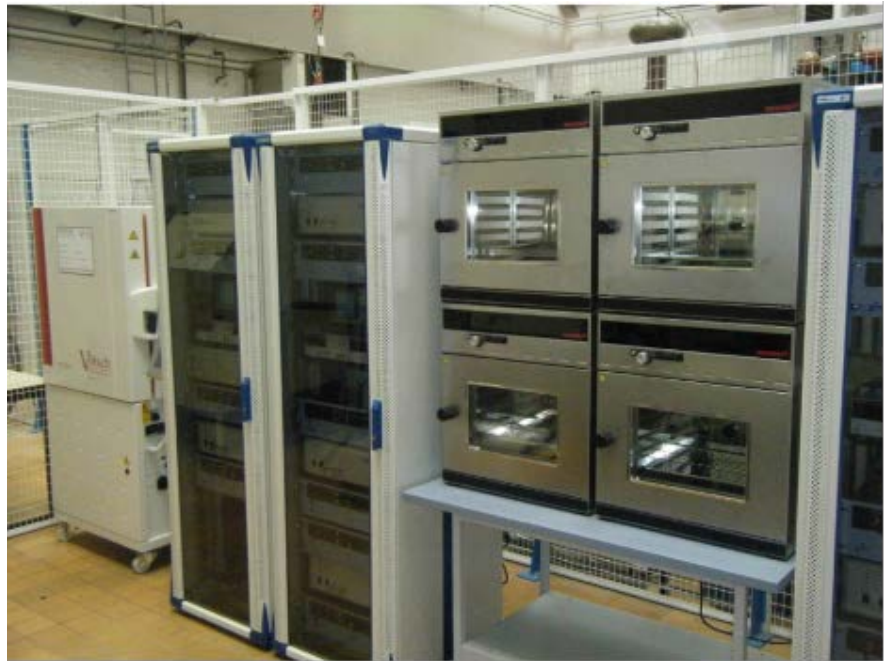
Figure 3. Experimental test-bench used to measure the lifetime under a PD.
