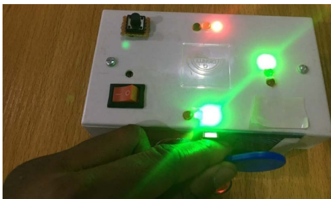
Figure 7. RFID tag is placed at the front of the RFID Reader.
