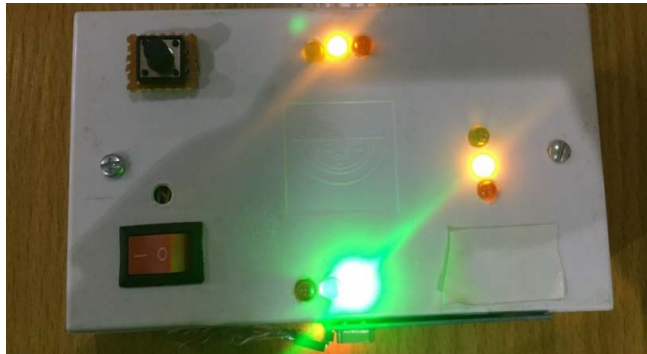
Figure 5. One traffic lane PASS, two on READY state.
