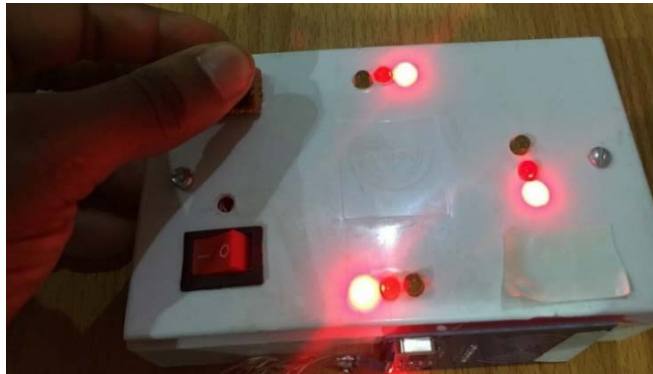
Figure 8. Switch pressed and held to activate the emergency mode.
