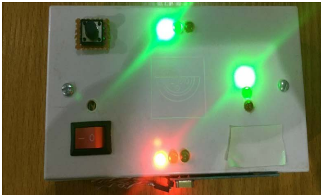
Figure 6. Two traffic lane PASS, one traffic lane on STOP state.
