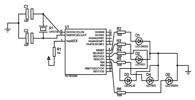
Figure 9. Circuit diagram of the moving message display board microcontroller.
