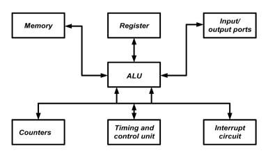
Figure 6. The basic arrangement of the internal structure of the microcontroller.
