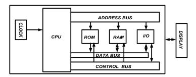
**Figure 1.** Block diagram of moving message display board designed with the incorporation of processor.
