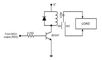
Figure 8. Switching transistor stage.
