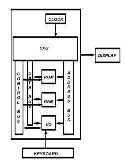
Figure 2. Block diagram of moving message display board designed with the incorporation of processor and a keyboard.
