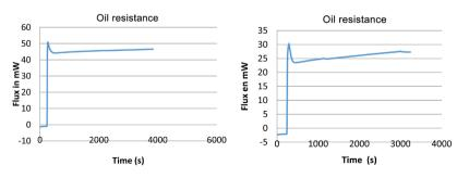
**Figure 5.** Attempted polymerization at 100°C (left) and 150°C (right) under oxygen of pumpkin oil in the presence of 3% irgacide.
