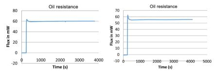
**Figure 4.** Attempted polymerization at 25°C (left) and 80°C (right) under oxygen of pumpkin seed oil in the presence of 3% irgacure.
