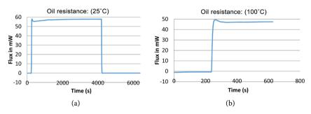
**Figure 1.** Attempted polymerization of pumpkin seed oil at 25°C (left: (a)) and 100°C (right: (b)) under nitrogen.
