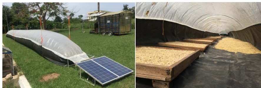
Figure 2. Set-up of drying experiment with elevated racks and maize on tarpaulin of SBD.
