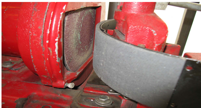
Figure 3. Bear Model 1420 abrasive surface and shoe attachment.
