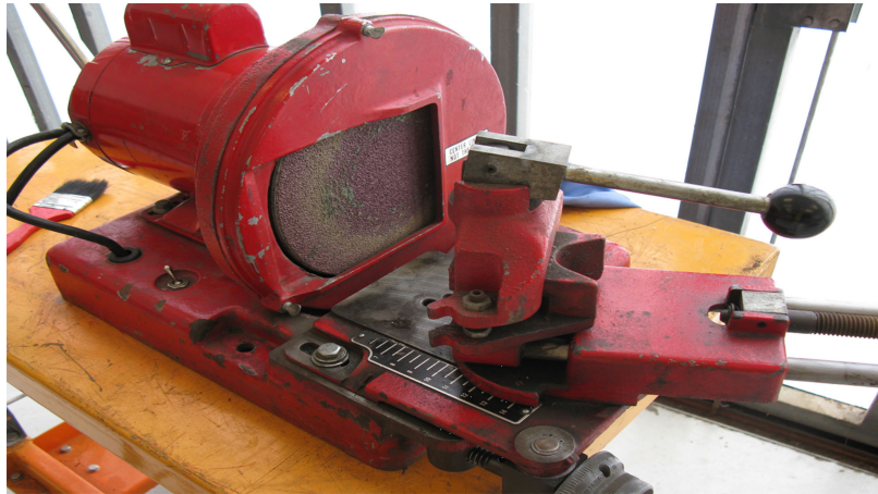
Figure 1. Bear Model 1420 automotive brake shoe grinder.
