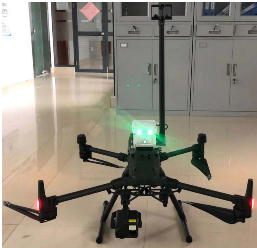
Figure 1. DJI M300 RTK equipped with meteorological detection instruments.
