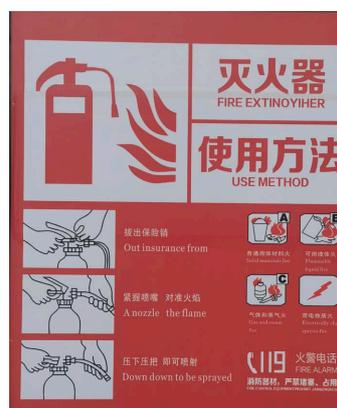
Figure 3. Fire extinguisher usage diagram
