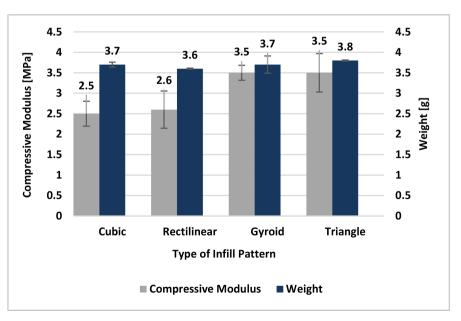
Graph 2. Comparison of compressive modulus of different patterns with 40% infill.
