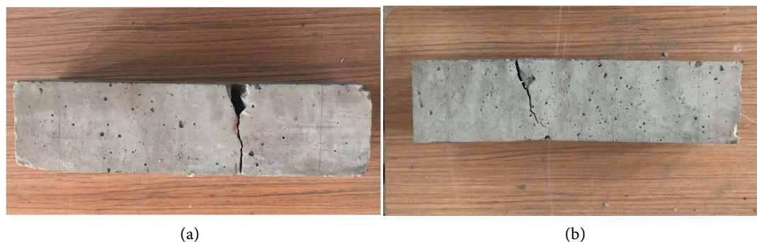
Figure 5. Fracture-resistant form. (a) The specimen without steel fiber; (b) The specimen with steel fiber.
