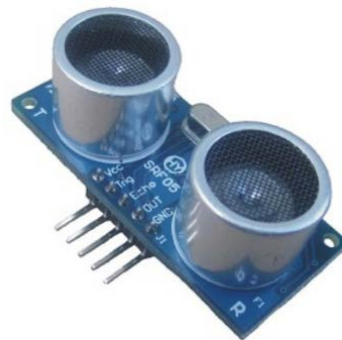
Figure 4. HC-SR04 ultrasonic distance measuring sensor.
