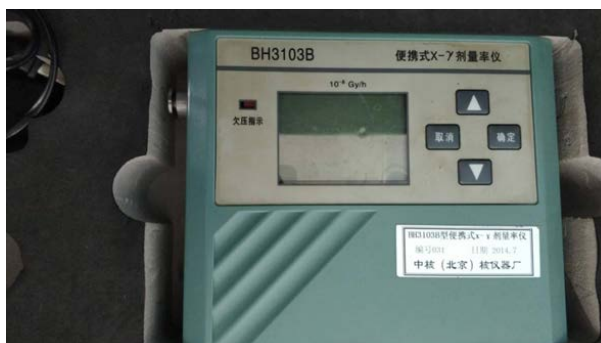
Figure 6. Control panel of dose-rate meter.
