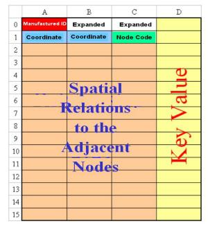
Fig. 3 Data contents stored in a multi-block tag
