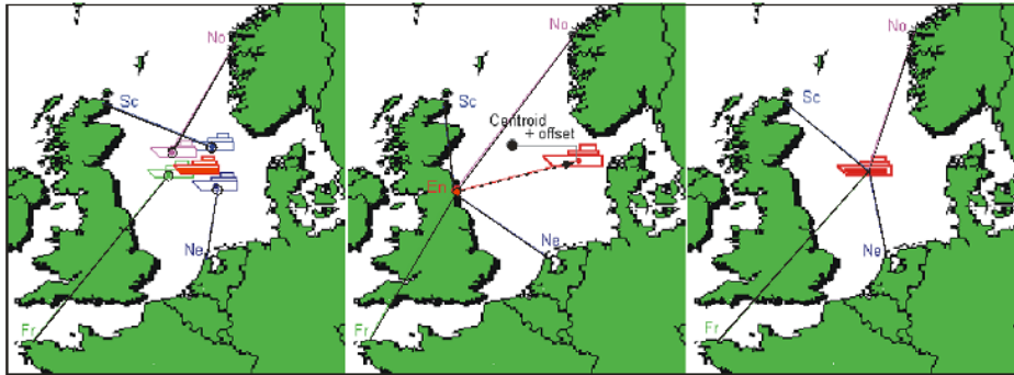
Fig. 3 The positioning methods using multi-DGPS references
