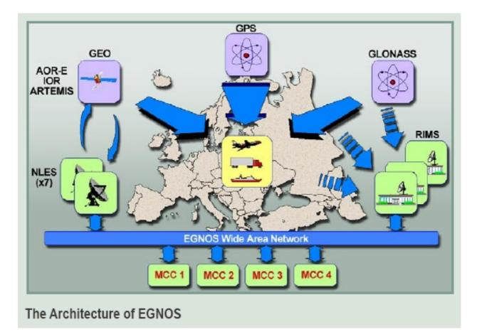
Fig. 8 EGNOS system (from an EC diagram) .
