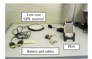
Fig. 10. Configuration of the low-cost code GPS (1Hz) system
