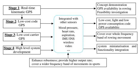
Fig. 9 Development roadmap of the prototype rowing tracking system
