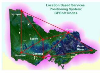
Figure 2 Victoria's GPSnet with LBS Positioning System stations generating a networked, statewide DGPS correction message which is then broadcast to users
