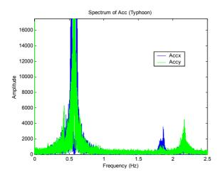
Figure 7 Zoom-in of the FFT spectrum of accelerometer.
