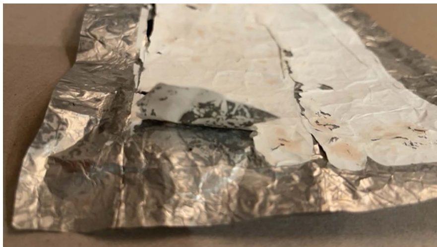
Figure 2. M1 (membrane prepared with 12% PVDF and 22% ZnO w/w). Note how membrane sticks to aluminum foil.
