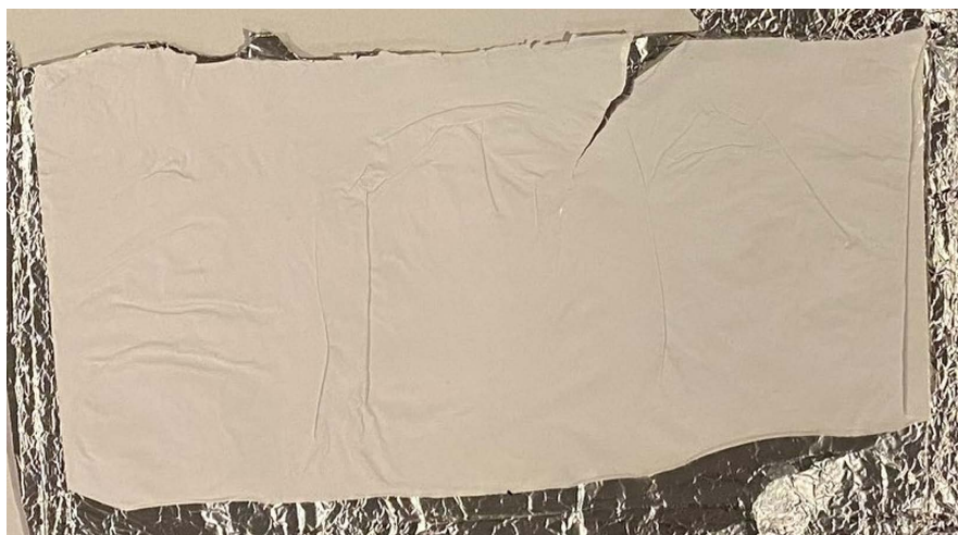
Figure 4. Electrospun membrane M3 (membrane with 22% PVDF and 12% ZnO w/w).
