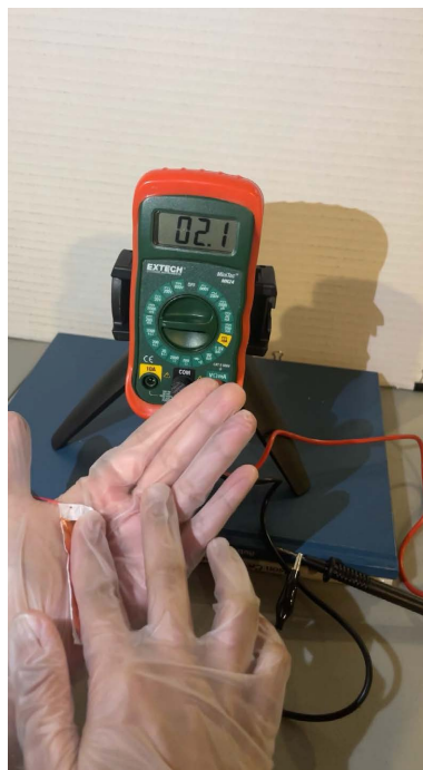
Figure 17. Non-zero voltmeter reading as prototype is subjected to mechanical stresses.
