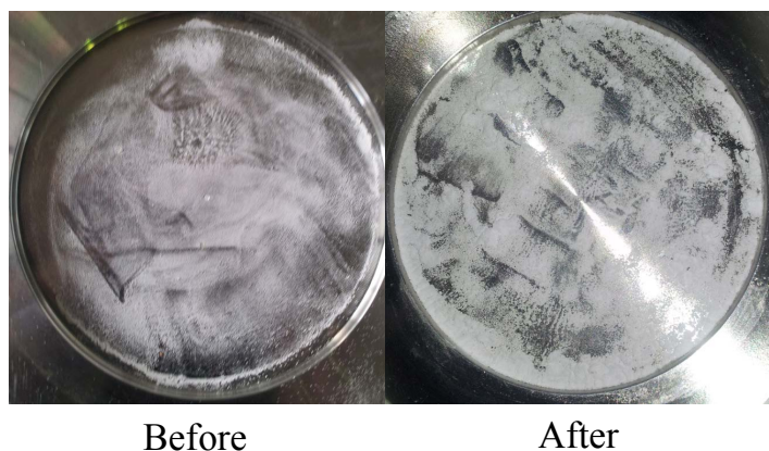
Figure 7. Photographs of the SrBr 2 sample before and after repeated cycles.
