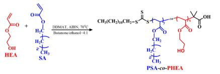
Scheme 2. Synthetic route of PHEA-co-PSA block copolymer.
