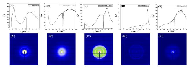
**Figure 5.** Iq<sup>2</sup>-q curves collected by SAXS and 2D SAXS patterns of PHEA-*b*-PSA ((A) and (A')), PHEA-*b*-PSA-*b*-PHEA ((B) and (B')), PSA-*b*-PHEA-*b*-PSA ((C) and (C')), P(HEA-*co*-SA) ((D) and (D')), and P(HEA-*grad*-SA) ((E) and (E')).
