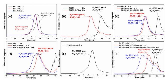
**Figure 2.** GPC traces curves of PSA (A), PHEA-*b*-PSA (B), PHEA-*b*-PSA-*b*-PHEA (C), PSA-*b*-PHEA-*b*-PSA (D), P(HEA-*co*-SA) (E), and P(HEA-*grad*-SA) (F) copolymer.
