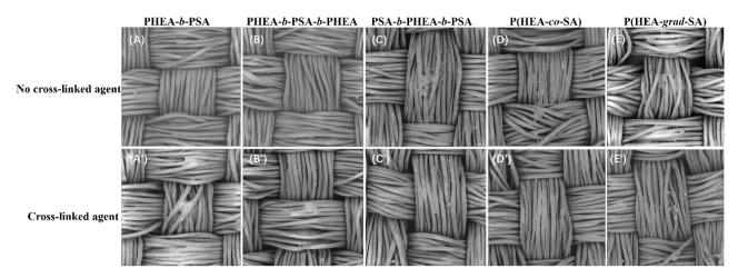
**Figure 4.** SEM images of PHEA-*b*-PSA, PHEA-*b*-PSA-*b*-PHEA, PSA-*b*-PHEA-*b*-PSA, P (HEA-*co*-SA), and P (HEA-*grad*-SA) copolymer coating polyester fabric. ((A), (B), (C), (D), and (E) represent the absence of a cross-linker. (A'), (B'), (C'), (D'), and (E') represent the addition of a cross-linker).
