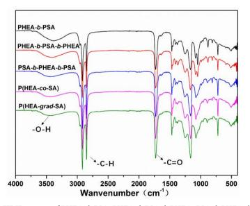
**Figure 1.** FT-IR spectra of PHEA-*b*-PSA, PHEA-*b*-PSA-*b*-PHEA, PSA-*b*-PHEA-*b*-PSA, P (HEA-*co*-SA), and P (HEA-*grad*-SA) copolymer.
