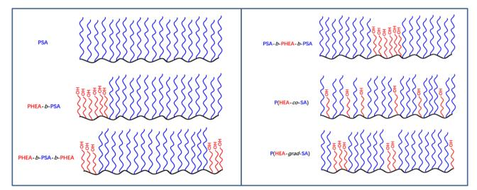
**Scheme 3.** The schematic diagram of targeted copolymers with different sequence structure. Abbreviated as PSA, PHEA-*b*-PSA, PHEA-*b*-PSA, PHEA-*b*-PSA, P(HEA-*co*-SA), and P(HEA-*grad*-SA).
