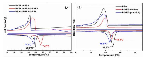
Figure 3. DSC scans for PSA, PHEA-*b*-PSA, PHEA-*b*-PSA-*b*-PHEA, PSA-*b*-PHEA-*b*-PSA, P (HEA-*co*-SA), and P (HEA-*grad*-SA) copolymer.
