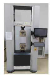
Figure 4. Universal test machine.
