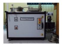
Figure 3. Pin on disc tribometer.
