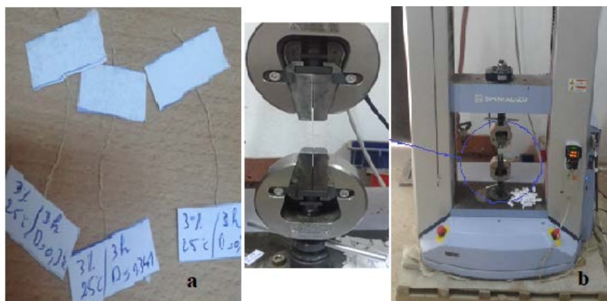
Figure 6. (a) Example of test pieces of luffa sponge fiber and (b) Traction machine.
